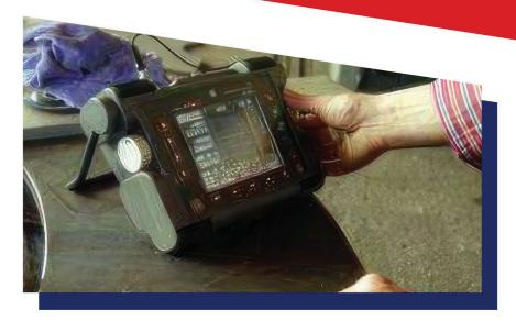
tions or to locate changes in material properties. The most commonly used ultrasonic testing technique is pulse echo, whereby sound is introduced into a test object and reflections (echoes) from internal.
